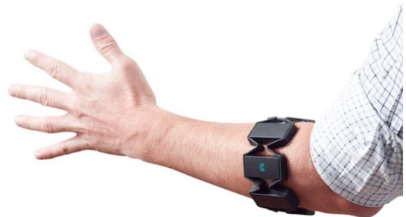
Figure 4: As demonstrated the proper way and positioning of the Myo armband if worn on the left forearm
